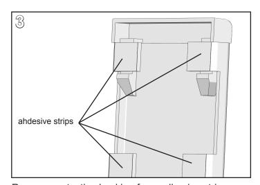
Remove protective backing from adhesive strips.
