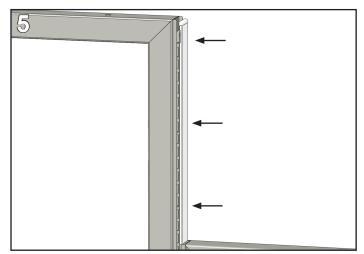
Apply light pressure along the length of the cover to ensure even adhesion.
