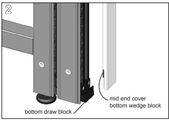
Place the bottom wedge block of the Mid End Cover over the bottom draw block of the connector.
