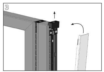
Pull up on the top draw block of the connector and rotate the Mid End Cover toward the connector so the wedge blocks are aligned.
