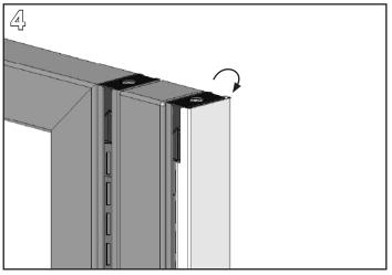
Drop the top draw block over both wedge blocks and tighten with a 1/4" Allen wrench. Note: Overtightening the top Allen screw may cause the end cover to bow.
