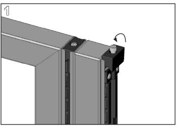
On the end of the connector, loosen the allen screw at the top of the with a 1/4" Allen wrench, pulling up on the draw block until it clears the top wedge block of the connector.
