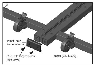
Bolt Joiner Plate into the threaded inserts on the bottom of each UltraFrame with a 3/8-16x1" flanged button head screw at each hole location in the Joiner Plate. Tighten securely using a 7/32" Allen Wrench/bit.
