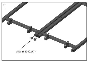
Connect UltraFrame with Panel Connector, Connector Post, or Corner Connector per connection product instructions. Lay frames down on a clean surface and remove glides at frame joint (save glides for future use).
