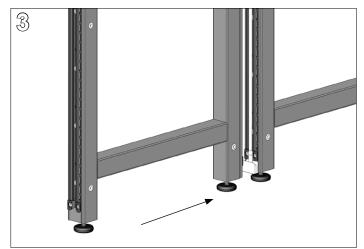
Align the taller frame with the shorter frame so the bottom draw block of the connector is below the bottom wedge block of both frames.
