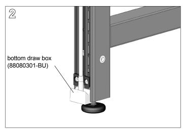
Loosen the Allen screw in the top of the connector using a ¼" Allen wrench until the bottom draw block of the connector clears the bottom wedge block of the frame.
