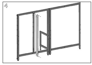
Repeat with the other Frame Spine half, installing it on the opposite face of the UltraFrame.
