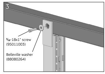
Fasten spine to frame with a Belleville washer, placed concave side against the tab, and a 1/16-18x1" cap screw using a 1/4" Allen Wrench/hex bit at the top and bottom of the Frame Spine tabs.
