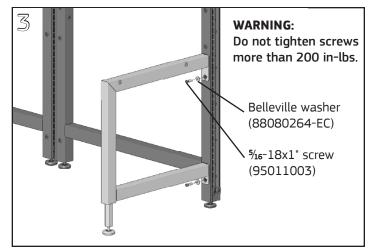
Fasten leg to frame/post with (2) Belleville washers placed concave side against the tab and (2) \$\frac{1}{6}-18x1"\$ cap screws using a \$\frac{1}{4}"\$ Allen wrench/hex bit. For legs with a glide adjust the glide up or down until the leg is level
