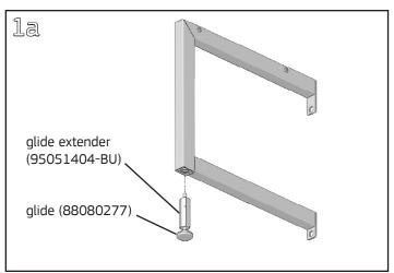
Leg with glide - locate CLG4 hardware pack (shipped separately) and install glide extender/glide assembly in the threaded hole in the bottom of the leg.
