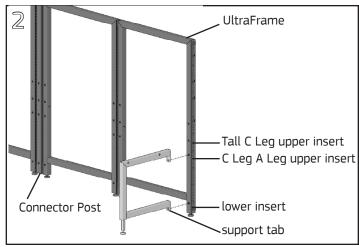
Align holes in the leg support tabs with the threaded inserts on the front or back face of an UltraFrame or Connector Post. On A Legs a plastic cap covers the top support tab. Remove the cap and replace after completing step 3.
