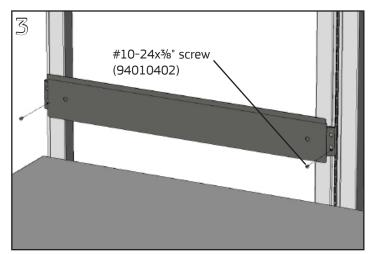
Install an additional #10-24x3%" Phillips panhead screw into the bottom keyslot hole of each hanger clip. Fully tighten all four hanger clips screws with a #2 Phillips screwdriver.
