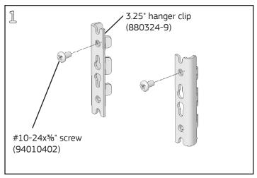
Install a #10-24x3%" Phillips panhead screw into the top of each hanger clip. Leave a  $\frac{1}{6}$ " gap between the screw and clip.
