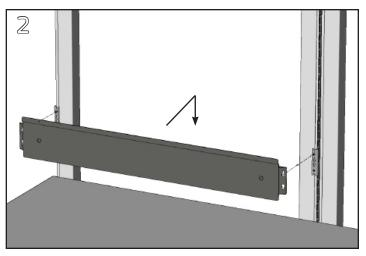
Install a hanger clip on the left and right side of the frame or panel with the screws at the top of each clip. Align the bottom of the keyslots in the bin rail with the heads of the #10-24 screws in the hanger clips. Slide the rail down over the screws to engage.
