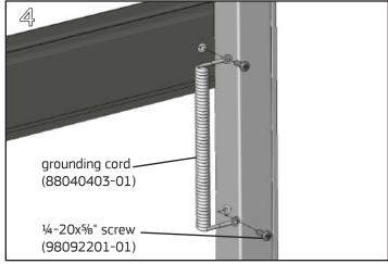
DISSIPATIVE FINISH ONLY - Attach one end of the grounding cord to the threaded insert in the back of the rail with a  $\frac{1}{4}$ -20x%" screw. Attach the other end of the cord to one of the frame's threaded grounding locations with an additional screw.
