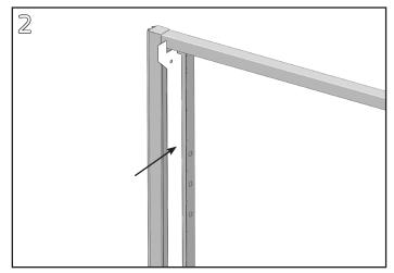
Before installing covers on the Vertical Utility Chase Housing, align the bottom of the divider with the bottom of the housing and adhere the divider to the back of the housing channel at the desired location.
