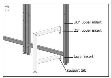
Align holes in the leg support tabs with the threaded inserts on the front or back face of an UltraFrame or Connector Post.
