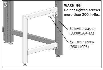
Fasten leg to frame/post with (2) Belleville washers placed concave side against the tab and (2) \$\frac{1}{16}-18x1" cap screws using a \$\frac{1}{4}\$" Allen wrench/hex bit. Adjust glide up or down until the leg is level when frame/leg assembly is in a stationary position.
