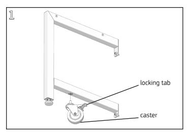
Leg with caster - locate caster (shipped separately) and lock it by pressing the tab near the top of the wheel. Install the caster in the threaded hole in the bottom of the leg.
