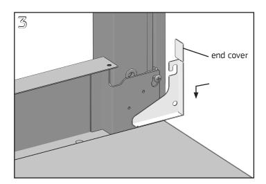
Slide end cover over and down onto upper hanger clip screw.
