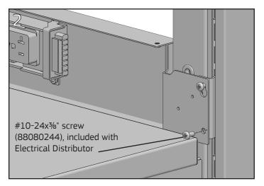
Using a **#2 Phillips screwdriver**, remove the lower hanger clip screw from the end of the distributor where end cover is to be installed. Loosen, but do not remove the upper hanger clip screw.
