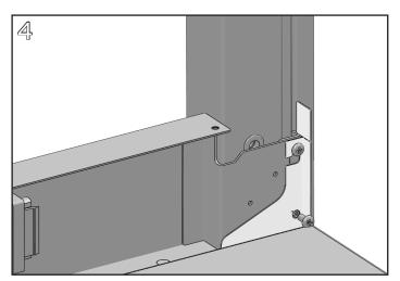
Reinstall lower hanger clip screw and tighten upper screw Reinstall face cover
