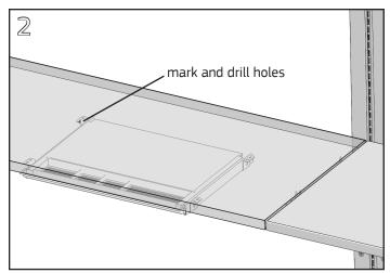
Hold closed pencil drawer in desired location on the underside of the surface. Mark the location of the slot in the top of each z-clip. Drill ¼" deep pilot holes at these locations using a ⅓" drill bit and cordless driver.
