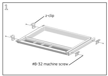
Attach the z-clips to the drawer slides with the small flange inboard in four locations with a #8-32 machine screw using a #2 Phillips screwdriver.
