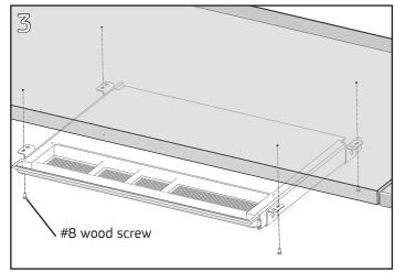
Fasten the pencil drawer to the surface with (4) #8 wood screws using a #2 Phillips screwdriver/drill with bit.
