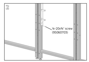
Align the bottom center end hole with the lower threaded insert on the inside of the UltraFrame tube. Fasten with (2) ¼-20 screws. Tighten both screws fully with a #2 Phillips screwdriver.
