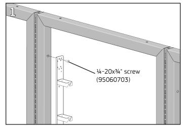
Align the center end hole in the Cable Duct with the top threaded insert on the inside of the UltraFrame tube. Loosely fasten with a ¼-20x¾" Phillips pan head screw.
