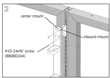
Align a set of 2" spaced holes in the top of the Cable Ring Duct with the top and bottom tapped holes in the hanger clip. The duct can be mounted inboard of the frame or center-mounted between frames. Fasten with (2) #10-24x3/6" Phillips pan head screws using a #2 Phillips screwdriver.
