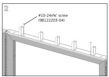
Fasten duct to the frame with a #10-24x%" Phillips pan head screw at each end using a #2 Phillips screwdriver.
