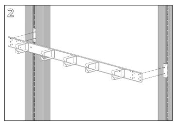
Align the set of holes closest to the ends of the Cable Ring Duct base with the center holes of the hanger clips.
