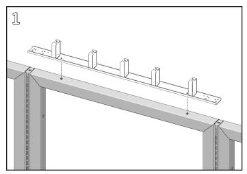
Center the Cable Ring Duct over the frame/frame run. Align the single centered slots near each end of the ring duct with the threaded inserts or knockouts in the top of the frame(s).
