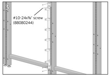
Repeat step two at the bottom of the Cable Ring Duct, and in the middle for 60" and 72" ducts.
