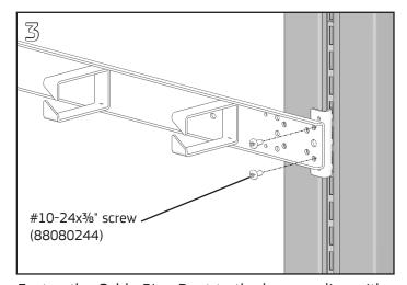
Fasten the Cable Ring Duct to the hanger clips with (2)  $\#10-24x^3\%$  Phillips pan head screws at each end using a #2 Phillips screwdriver.
