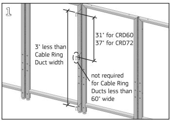
Install two or three hanger clips on one side of the frame depending on Cable Ring Duct width.
