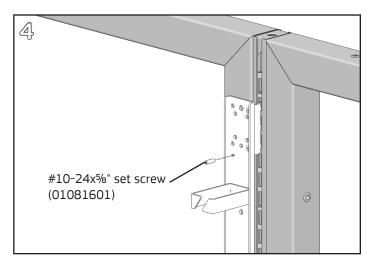
Install a #10-24x%" set screw into a tapped hole near the top clip and tighten with a <sup>3</sup>/<sub>32</sub>" **Allen wrench** until the set screw tip pushes against the UltraFrame. Repeat at bottom clip location.
