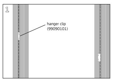
Install a hanger clip on the left and right side of the frame at the designated mounting height.
