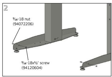
Install a 1/16-18x1/2" cap screw through the back hole of each glide base and fasten with a 1/16-18 nylock nut on the outward side of the base. Tighten fully with a 1/4" Allen wrench and 1/2" wrench or nutdriver
