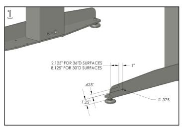
Drill two 3/8" diameter holes through the side of each glide base at the location shown.
