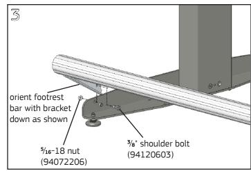
Align holes in end of footrest bar with the front hole in each glide base. Fasten each end with a shoulder bolt and 1/6-18 nylock nut. Tighten fully with a 3/16" Allen wrench and 1/2" wrench or nutdriver. Footrest can be rotated forward (shown) or back.
