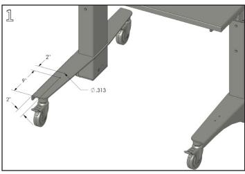
Drill two 1/16" diameter holes through the top of each caster base at the location shown.
