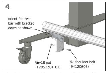
Align holes in end of footrest bar with the middle hole in each footrest bracket. Fasten each end with a shoulder bolt and 1/16-18 nylock nut. Tighten fully with a 3/16" Allen wrench and 1/2" wrench or nutdriver. Footrest can be rotated forward (shown) or back.
