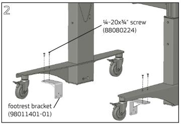
With the flanges on the footrest brackets facing inward, align the two holes in the brackets with the drilled holes in the caster bases. Fasten each bracket with (2) ½-20x¾" button head screws using a 5/32" Allen wrench.
