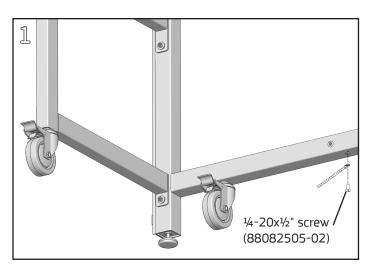
Locate the threaded insert or hole at the center underside of the bottom tube of the UltraFrame. Fasten ring terminal of Ground Chain to frame with a 4-20x Phillips pan head screw using a **#2 Phillips screwdriver**.
