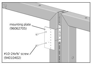
Attach a mounting plate to each hanger clip using (2) #10-24x<sup>3</sup>/<sub>8</sub>" Phillips pan head screws using a **#2 Phillips screwdriver**.
