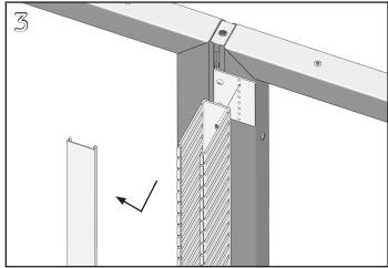
Remove the duct cover to access the slots in the back of the duct base. Align a slot at each mounting plate location with one of the tapped holes in the plate.
