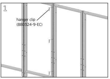
Install a hanger clip in one side of the frame at the top, near the middle, and at the bottom where the Cable Duct will be located.
