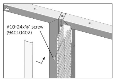
Fasten duct to each plate with a #10-24 screw using a **#2 Phillips screwdriver**. Replace cover after cable lay-in is complete.
