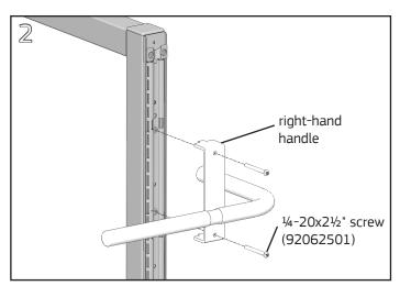
Align holes in right-handed handle with the threaded inserts and fasten with (2) ¼-20x2½" socket button head cap screws using a 5/32" Allen wrench.
