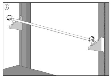
Slide the material spool (not provided) onto the rod. Place the rod between the brackets in one of the notches with the washers outboard of the bracket. Securely tighten thumbscrew to prevent spool from disengaging.
