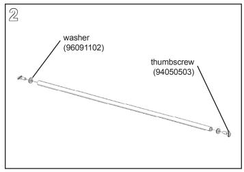
Place a  $^{1}/_{4}$ " flat washer on each  $^{5}/_{16}$ - $18x^{3}/_{4}$ " thumbscrew and loosely fasten a thumb screw to each end of the spool holder rod/spindle.
