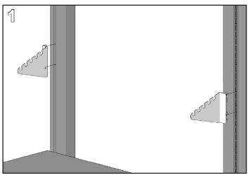
With notched edge of bracket up, engage the lefthand bracket into the left side of the frame. Repeat with right-hand bracket on the right side. Ensure that the brackets are at the same height and are firmly seated in the hanger frame slots.
