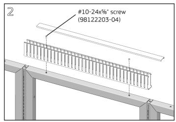
Remove cover to access slots in the base. Align two of the slots with the threaded inserts or knockouts in the top of the UltraFrame. Fasten with a #10-24x%" Phillips pan head screw at each insert using a #2 Phillips screwdriver. Replace cover after cable lay-in is complete.
