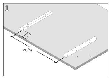
Determine position for Tote Bearer on underside of surface. The front holes of the drawer bearers should be positioned 3" from the front edge of the surface and spaced 20 \(^3\/\_6\)" apart. Mark hole locations using drawer bearers.
