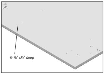
Using a %" drill bit and cordless drill, drill %" deep holes at the marked locations.
