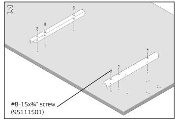
With open end of Tote Bearers facing the front of the surface, attach each bearer with (3) #8-15x¾" Phillips flathead screws using a #2 Phillips bit and cordless drill
