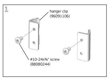
Install a #10-24x3/6" Phillips pan head screw into each hanger clip at opposite ends, leaving a gap between the screw and clip.
