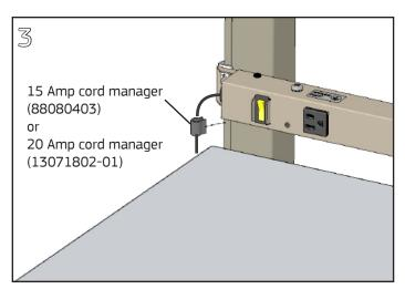
Place cord manager around plug strip cord and push into hanger frame slots to manage cord.
