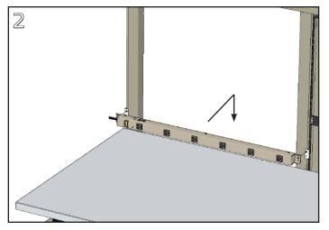
Install a hanger clip on the left and right side of the frame or panel with the screws at the top of each clip. Align the bottom of the keyslots in the plug strip with the heads of the #10-24 screws in the hanger clips. Slide the power strip down over the screws to engage.
