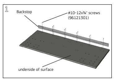
On underside back edge of surface, align the backstop with pre-drilled holes in surface as shown in the above image. Attach with #10-12x¾" screws provided. Tighten all screws securely with a #2 Phillips screwdriver.
