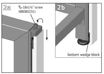
Loosen the Allen screw at the top of the End Cover with a ¼" **Allen wrench** (2a) until the bottom draw block of the end cover clears the bottom wedge block of the UltraFrame (2b).
