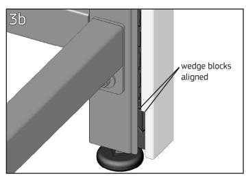
Tighten the Allen screw in the top of the Panel End Cover (3a), ensuring that the end cover bottom draw block captures the UltraFrame bottom wedge block (3b). *Note: Overtightening the top allen screw may cause the end cover to bow.*
