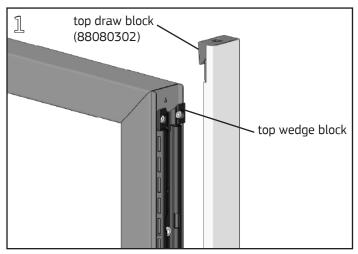
On the end of the frame, place the Panel End Cover top draw block over the top wedge block of the UltraFrame.
