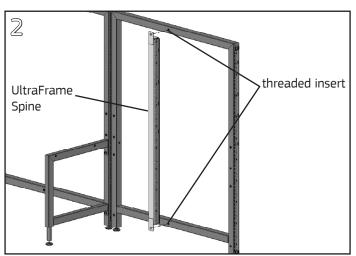
Align the hole in the top and bottom tab of one half of the Frame Spine with the threaded inserts in the top and bottom of the UltraFrame. Orient the hanger frame slots of the frame spine on the right-hand side of the threaded inserts of the UltraFrame.
