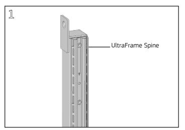
Identify top end of Frame Spine by locating the small "T" cut through the hanger frame on each frame spine half. Orient this end up.
