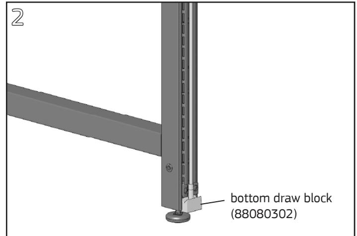
Loosen the Allen screw in the top of the Panel Connector using a ¼" Allen Wrench bit until the bottom draw block clears the bottom wedge block of the frame.
