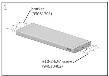
Lay Task Light with the lens side down on a clean surface. Position mounting brackets on the ends of the light with the top flanges outboard. Fasten each bracket to the light with (3) #10-24x¾" Phillips pan head screws (provided with light) using a #2 Phillips screwdriver.
