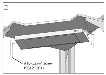
Install the Corner Shelf per instructions. Align the light brackets with the four pre-drilled holes in the underside of the shelf. Fasten with #10-12x3/4" screws using a **cordless drill** and **#2 Phillips bit**.
