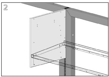
With the screws to the inside, install the end panels on the left and right sides of the frame. Ensure the panels are firmly seated in the hanger frame slots and use a tape measure to verify both panels are at the same height.
