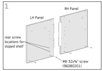
Install two #8-32x3%" Phillips pan head screws into the lower holes on each end panel leaving an 1%" gap between the panel and screw. To install the shelf in a sloped position, install the rear screw in one of the higher positions of the end panel.
