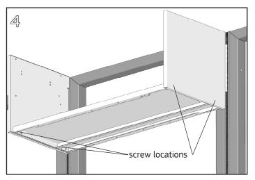
Rotate the shelf down toward the back until the straight slots in the sides of the shelf slide over the rear panel screws. Tighten all four screws with a #2 Phillips screwdriver.
