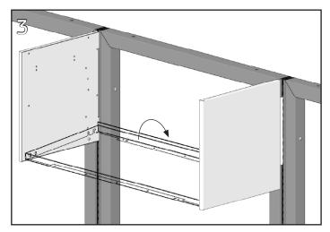
For a flat shelf, orient the lip toward the back and engage the dog-leg slots in the sides of the shelf with the front screws in the end panel. If installing in a sloped position, the shelf lip should be at the front.
