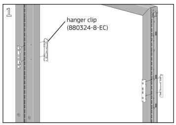
Install two hanger clips at the same height, one on the front and the other on the back of the hanger frame, on both the left and right sides of the frame. Ensure the clips are firmly seated in the slots.
