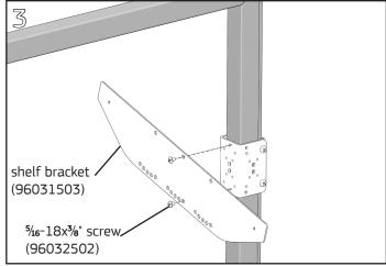
Determine the shelf position and angle. With shelf bracket weldnuts facing outward, fasten each shelf bracket to a saddle bracket with (2) \(^5\)16-18x\(^3\)8" button head cap screws using a \(^3\)16" Allen wrench.
