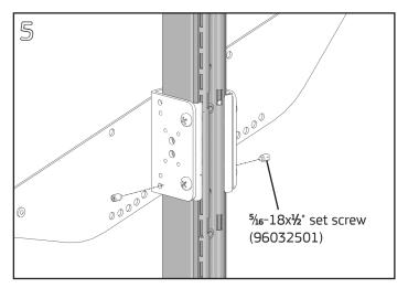
Secure each saddle bracket to the vertical tube of the frame by installing (2)  $\frac{1}{16}$ - $\frac{18x}{2}$ " nylon tip set screws, one on the front and one on the back of the saddle bracket, using a  $\frac{1}{32}$ " Allen wrench.
