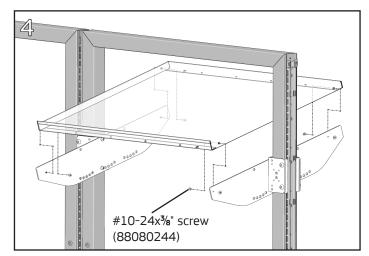
Position shelf between the shelf brackets, aligning the holes in the sides of the shelf with the weldnut holes in the shelf brackets. From beneath the shelf, fasten to each bracket with (2) #10-24x3/8" Phillips pan head screws using a #2 Phillips screwdriver.
