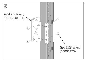
Place a saddle bracket over each pair of clips. Fasten the bracket to the clips with (4) \%-18x\%" Phillips pan head screws using a #3 Phillips screwdriver.
