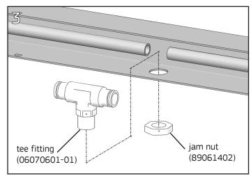
Install tee fitting in open hole and connect each end to the cut tubing. Fasten tee with jam nut.
