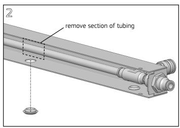
Remove the plug from the location where the Quick Disconnect Fitting is to be installed. Cut and remove approximately 1" of tubing at this location using a **Tube Cutter**.
