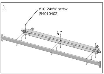
Remove the back of the Air Strips by unfastening the #10-24x%" Phillips pan head screws using a #2 Phillips screwdriver.
