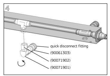
Thread Quick Disconnect Fitting onto end of tee fitting. Reassemble Air Strip back.
