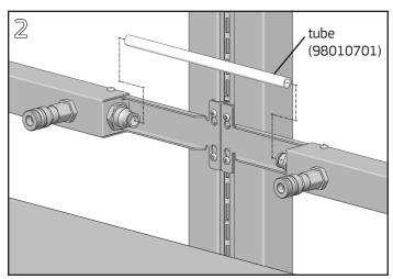
Insert tube ends into the end fitting of each Air Strip.
