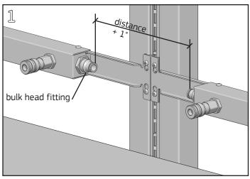
Measure distance between adjacent Air Strip bulkhead fittings. Add approximately 1" to this measurement and cut ½" tube to length using **Tube Cutter**.
