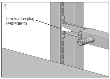
Insert Termination Plug into the last Air Strip end fitting of the run.
