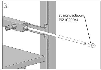
Cut tube to length if required with the **Tube Cutter**. Push end of tube into straight adapter.
