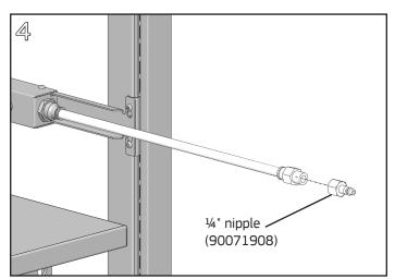
Connect the straight adapter to building air supply, or assemble the  $\frac{1}{4}$ " quick disconnect nipple to the straight adapter for source connection.
