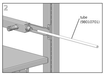
Insert the  $\frac{1}{2}$ " tube provided into the end fitting of the Air Strip at the beginning of the run.
