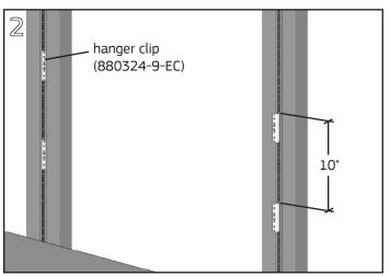
Install two hanger clips on the right side of the frame with a spacing of 10" between the tops of the clips. Repeat on the left side at the same heights.
