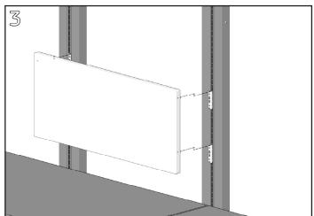
Align screws in back of the board with the notches in the tops of all four hanger clips. Slide the tack-board down over the clips to engage screw heads.
