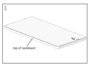
If necessary, loosen the screws in the back of the tackboard so there is a  $\frac{3}{16}$  gap between the board and screw head using a #2 Phillips screwdriver.
