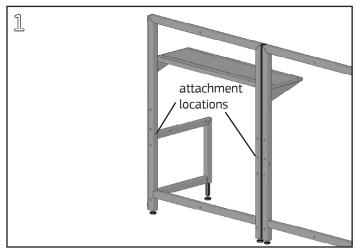
Threaded insert attachment locations for the Common Point Ground plate can be found on the inside faces of the vertical tubes of UltraFrames and Riser Frames. There is one on the left and one on the right side of each frame.
