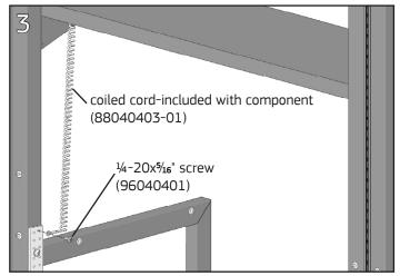
Route the coiled cords which are attached to the dissipative finish components to the Common Point Ground plate. Fasten the ring terminal on the cord to the plate with a 1/4-20x5/16" Phillips pan head screw. Up to twelve coil cords can be attached to the plate.
