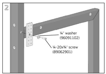
Align the center hole in the plate with the threaded insert in the frame and fasten with a  $\frac{1}{4}$ " flat washer and  $\frac{1}{4}$ -20x $\frac{3}{4}$ " Phillips pan head screw using a #2 Phillips screwdriver.
