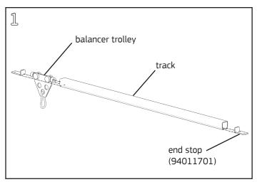
Install Cantilever Light Brackets with or without Task Light per installation instructions. Slide balancer trolly into track. Insert an end stop, flange first, into each end of the track.
