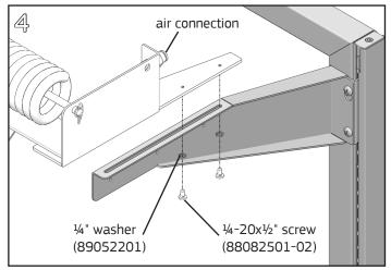
Fasten each Tool Traveler support bracket to the slots in the top of the Cantilever Light Brackets with (2) ¼-20x½" Phillips pan head screws and (2) ¼" external tooth lock washers using a **#2 Phillips** screwdriver. Connect to building air supply via straight adapter on the back of the support bracket.
