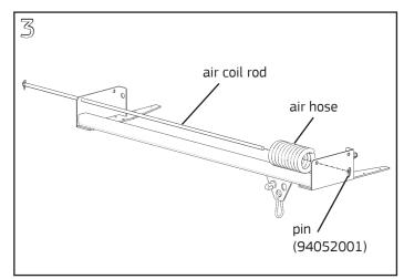
Remove the pin from one of the ends of the air coil rod. Align rod with the hole in the support bracket above the track and insert unpinned end. Place the coiled air hose on the rod and then insert through the hole in the other support bracket. Reinsert pin and connect air hose to tool travel car and air fitting in support bracket.
