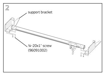
Center track between support brackets. Align the holes in the end stops with the two holes in the bottom of the support brackets, in either the front or rear position. Fasten each end with (2) ¼-20x1" Phillips pan head SEMS screws using a #2 Phillips screwdriver.
