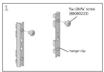
Install a 5/16-18x3/6" Phillips pan head screw into each hanger clip at opposite ends, leaving a 3/16" gap between the screw and clip, using a #4 Phillips screwdriver.
