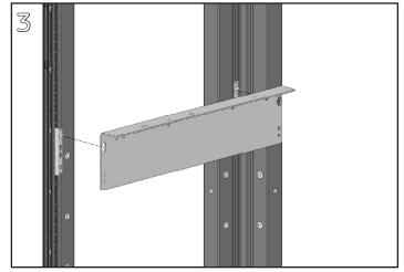
Align the large hole in the center of the keyslots in the Frame-mount Surface Support bracket with the heads of the  $\frac{1}{100}$ -18 screws in the hanger clips.
