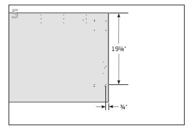
Flip the surface to be mounted to the bracket upside down. Locate the hole as indicated above for the pin.
