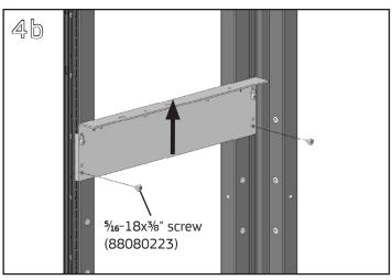
B/C Height Module – Slide the support up and install a 5/16-18x3/8" Phillips pan head screw in the lower clearance hole near the bottom of the support on each end. Fully tighten all four hanger clips screws with a #4 Phillips screwdriver.
