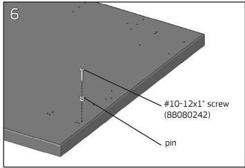
Install a pin at the required location with a #10-12x1" screw using a **cordless drill and #2 Phillips bit**. Install additional surface supports and surface mounting hardware as needed on the other end of the surface
