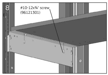
Install a #10-12 $x^3$ 4" screw into the hole near the back of the support, and also near the front of the support in front of the pin using a **cordless drill** and a #2 Phillips bit.
