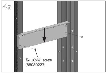
Lab Height Module – Slide the support down and install a 5/16-18x3/8" Phillips pan head screw in the upper clearance hole near the bottom of the support on each end. Fully tighten all four hanger clips screws with a #4 Phillips screwdriver.
