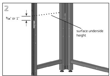
Install a hanger clip on the left and right sides of the frame with the screws at the top of each clip. The top of the clip should be mounted 5/16" below the desired surface underside height when used with Lab height module products (LULL, LUSA, LUSC, LUSB), and 1" below when used with B Support/C Leg height module products (WBL/R, WBEL/R, WSL/R). Ensure that the clips are firmly seated in the slots.
