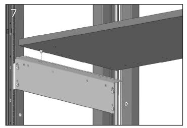
Flip the surface over and align the pin with the large diameter hole near the front of the Frame-mount Surface Support Bracket.
