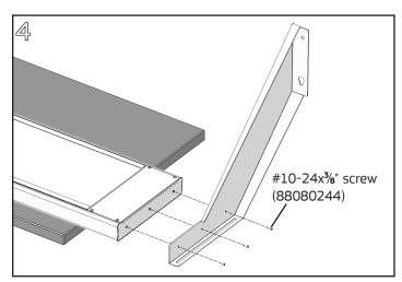
Align the holes in the left side of the light with the three holes in the left-hand Cantilever Light Bracket. Install (3) #10-24x¾" Phillips pan head screws with a #2 Phillips screwdriver. Repeat for the right-hand Cantilever Light Bracket.
