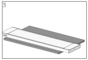
Lay the Task Light upside down on a clean, smooth surface (lamps facing upward). With the sides overhanging the surface, install lens as required per Task Light instructions.
