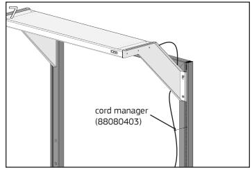
Place cord manager around Task Light cord and push into hanger frame slots to manage cord.
