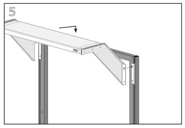
Flip light/bracket assembly over and align the bottom of the keyslots in the Cantilever Light Brackets with the heads of the 5/16-18 screws in the hanger clips. Slide the light/bracket assembly down over the screws to engage.
