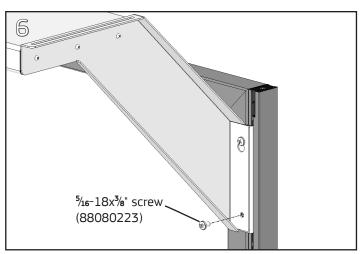
Install an additional 5/16-18x3/8" Phillips pan head screw in the hole below the keyslot on each Cantilever Light Bracket. Fully tighten all four hanger clips screws with a #4 Phillips screwdriver.
