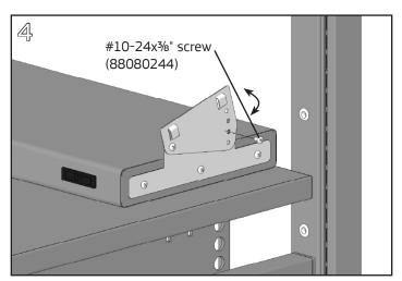
Pivot the bracket until the rear hole in the mounting bracket aligns with one of the angle-setting holes in the adjustable bracket. Fasten with an additional #10-24x3/8" Phillips pan head screw and tighten both screws with a #2 Phillips screwdriver. Repeat step 3 and 4 on opposite end of the Task Light.
