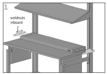
Install lens as required per Task Light instructions. Gently rest the light on a clean, smooth surface in the upright position. The mounting brackets are not handed, but when attached, the weldnuts at the top of the bracket must face inboard of the light.
