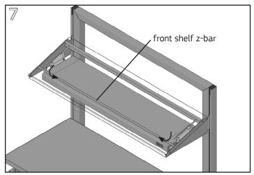
Gently bend the front tops of the spring bars inward and engage them over the front flange on the underside of the shelf. Straighten bars and position the light under the shelf.
