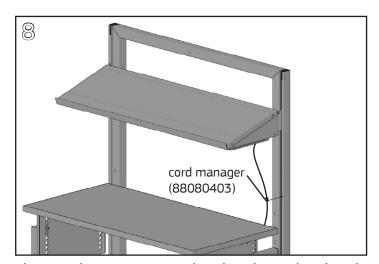
Place cord manager around Task Light cord and push into hanger frame slots to manage cord.
