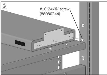
Align the three holes in the mounting brackets with the holes in the end of the Task Light and secure with three #10-24x3/8" Phillips pan head screws using a #2 Phillips screwdriver. Repeat on opposite end of Task Light.
