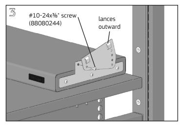
Loosely fasten adjustable bracket to the outside face of the mounting bracket using a #10-24x¾" Phillips pan head screw in the front hole. The lances on the adjustable bracket must face outward.
