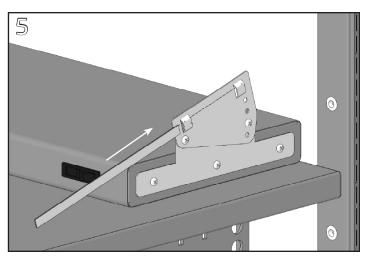
Insert two spring bars per side through the lances in the adjustable brackets. Various spring bar lengths are provided depending on shelf style.
