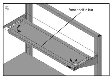
Gently bend the front tops of the spring bars inward and engage them over the front flange on the underside of the shelf/cabinet. Straighten bars and position the light under the shelf.
