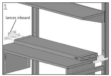
Install lens as required per Task Light instructions. Gently rest the light on a clean, smooth surface in the upright position. The mounting brackets are not handed, but when attached, the lances at the top of the bracket must face inboard of the light.
