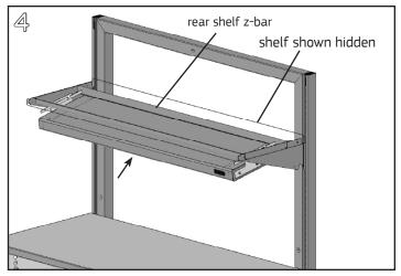
Under the installed shelf or cabinet, place the back tips of the spring bars over the rear flange or z bar on the underside of the shelf. Slide the light along the spring bars toward the back of the shelf/cabinet.
