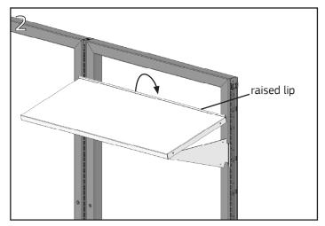
For a flat shelf, position the raised lip of the shelf at the back. For a sloped shelf, position the lip at the front. Align the front tips of the shelf brackets with the inside faces of the shelf sides. Rotate the shelf back until it drops over the back of the shelf brackets.
