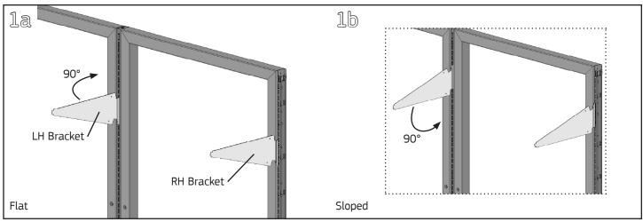
Engage the brackets in the left and right sides of the frame or frame span as shown above for either a flat or sloped mounting configuration. Ensure the brackets are firmly seated in the hanger frame slots and use a tape measure to verify both the right and left-hand brackets are at the same height.
