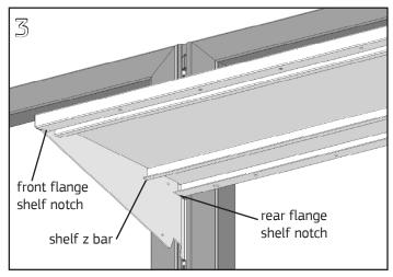
On the underside of the shelf, ensure that both right and left brackets are engaged in the notches of the shelf flanges and between the shelf z bars.
