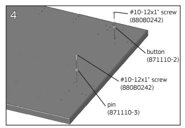
Install each pin and button at the required location with a #10-12x1" screw using a **cordless drill and #2 Phillips bit.** Tighten the pin fully, but leave an '%" gap between surface and underside of button. Install additional surface supports and surface mounting hardware as needed on the other end of the surface
