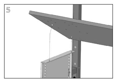
Flip the surface over and align the button with the large end of the keyslot near the back of the Surface B Support. Push the surface back while rotating down so the pin aligns with the large diameter hole near the front of the Surface B Support.
