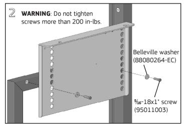
Align the selected height holes in the support with the threaded inserts on C Leg. Fasten Surface B Support to the C Leg with (2) Belleville washers placed concave side against the Surface B Support Bracket and (2) \% 16-18x1" cap screws using a \%4" Allen Wrench/Hex Bit.
