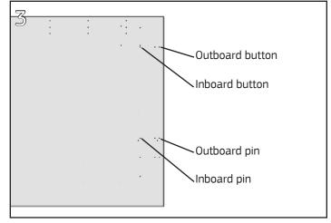
Flip the surface to be mounted to the bracket upside down. Locate holes as indicated above for the pin and button. If the C Leg with Surface B Support is mounted on the same frame as the surface, use the "Inboard" position. If C Leg is mounted on a frame adjacent to the surface, use the "Outboard" position.
