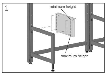
Determine the required surface height. The top set of holes in the side of the Surface B Support Bracket will locate the top of the bracket 25%" from the floor when mounted on a CLM, or 30%" from the floor when mounted on a CLT. Additional hole locations are spaced in 1" increments for a total height adjustment range of 10".
