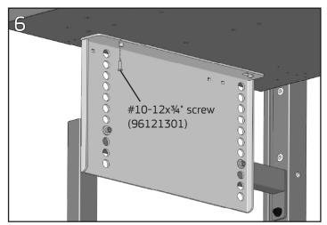
Fully tighten the button and install a #10-12x3/4" screw into each of the remaining holes in the top of the Surface B Support (WB has one hole, WBE has two holes).
