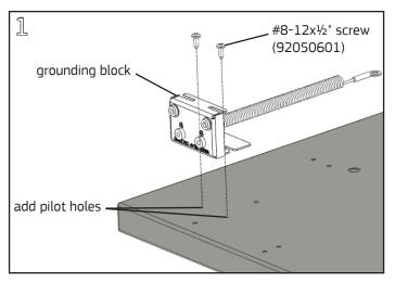
Flip the surface upside down. Place Wrist Strap Grounding Block in desired mounting position and mark the mounting hole locations. Using a **drill bit** and cordless drill, drill two pilot holes approximately ½" deep. With the coiled cord facing the rear of the surface, mount Grounding Block in the pilot holes using two #8-12x½" Phillips pan head screws.
