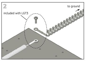
Attach the other end of the coiled ground cord to the ESD Laminate Grounding Terminal (installed per LGT3 instructions) using the screw and washers included with the terminal. Ensure the terminal is attached to an appropriate ESD ground path.
