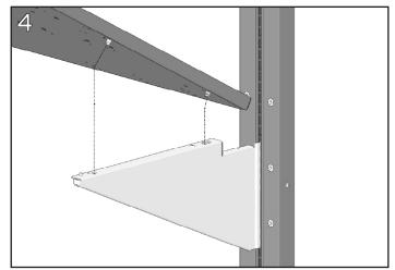
Flip the surface over and align the button with the large end of the keyslot near the back of the Cantilever Support. Push the surface back while rotating down so that the pin aligns with the large diameter hole near the front of the support.
