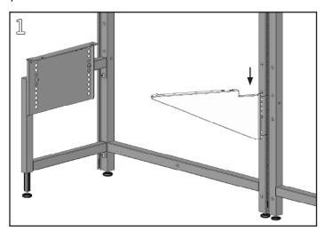
Rotate the Cantilever Support at an angle inboard of the frame. Align with hanger frame slots in the side of the frame at appropriate height. Push the support down to securely seat in the slots. Surfaces 72" and wider require an additional support at frame joint.
