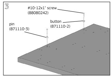
Install each pin and button at the required location with a #10-12x1" screw using a **cordless drill** and a **#2 Phillips bit**. Tighten the pin fully, but leave a 1/8" gap between the surface and underside of the button. Install additional surface supports and surface mounting hardware as needed on the other end of the surface
