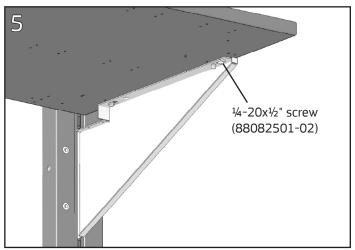
Fully tighten the button. Level the surface by adjusting the  $\frac{1}{4}$ -20x½" Phillips pan head screw which has been preinstalled near the front of the Cantilever Support.
