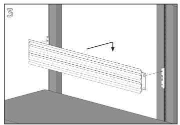
Align the bottom of the keyslots in the slatwall rail with the heads of the #10-24 screws in the hanger clips. Slide the rail down over the screws to engage.
