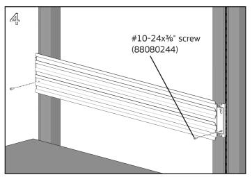
Install an additional #10-24 screw into the bottom hole of each hanger clip. Fully tighten all four hanger clip screws with a #2 Phillips screwdriver.
