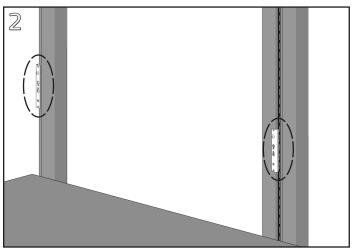
Install a hanger clip on the left and right side of the frame or panel with the screws at the top of each clip. Ensure the clips are at the same height and firmly seated in the hanger frame slots.
