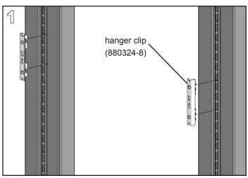
At designated mounting height, install hanger clips on left and right sides of the frame. Ensure the clips are at the same height and firmly seated in the hanger frame slots.
