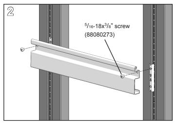
Align top hole in Tote Rail with the top threaded hole in the hanger clip. Fasten rail to clips with one 5/16-18x3/8" Phillips pan head screw per side using a #4 Phillips screwdriver.
