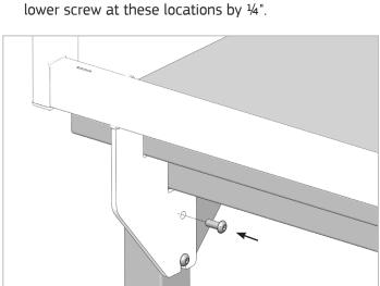
3. Reinstall the upper screws and tighten all four gusset plate screws securely using a 3/16" hex bit and driver or Allen wrench.
