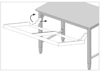
2. Align the notches on the Riser Frame blades with the lower screws in the table gusset plates and rotate the frame up to vertical while resting on these screws.
