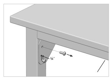
1. On the back side of the assembled 4-Legged Table, remove the upper screw only in the gusset plate attached to the vertical tube on the left and right sides of the table using a 3/16" hex bit and driver or Allen wrench. Then loosen, but do not remove, the lower screw at these locations by 1/4".
