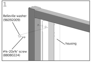
Align the large holes in the 2" side of the housing channel with the threaded inserts on the inside of the Riser Frame tube. Fasten housing to frame at the top and bottom with (2)  $\frac{1}{4}-20x\frac{3}{4}$ " socket button head screws and (2) Belleville washers using a  $\frac{5}{32}$ " Allen wrench.
