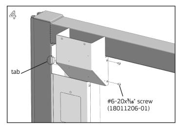
Align slot in the side of the routing cover with the tab on the housing channel. Slide routing cover over tab and fasten with (2) #6-20x<sup>3</sup>/16" Phillips pan head screws using a #2 Phillips screwdriver.
