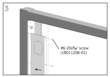
Align tabs on cover with slots in the short flange of the housing. Slide cover into slots and align holes in the cover flange with the holes in the housing. Fasten cover to housing with (7) #6-20x3/16" Phillips pan head screws using a #2 Phillips screwdriver.
