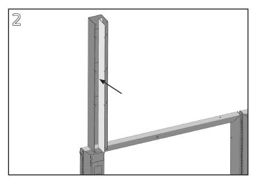
Before installing covers on the Vertical Utility Chase Extender, align the bottom of the divider with the bottom of the housing and adhere the divider to the back of the housing channel at the desired location.
