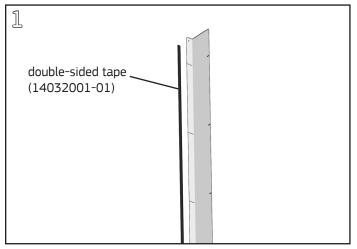
Apply the double-sided tape to the back flange of the divider.
