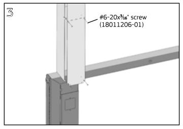
Route utilities through extender. Attach extender cover using #6-20x¾6" Phillips pan head screws using a #2 Phillips screwdriver.
