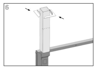
Attach Vertical Utility Chase Extender to ceiling structure (hardware not provided). Place ceiling trim on chase extender and align with finished ceiling.
