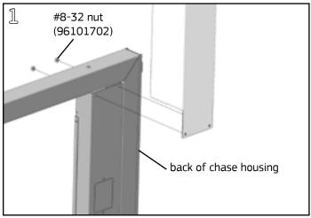
Align the threaded studs in the bottom of the Vertical Utility Extender channel with the knockout clearance holes in the back of the Vertical Utility Chase Housing. Fasten with (2) #8-32 lock nuts using a %" nutdriver.
