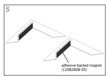
Apply adhesive-backed magnets to the ceiling trim plates as shown.
