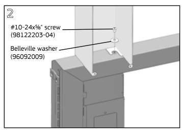
Secure the bottom flange of the extender channel to the frame by installing a #10-24x%" screw and Belleville washer in the threaded insert or knockout on the top of the frame using a #2 **phillips screw driver**. If installing on a 30" wide frame, there will be two inserts or knockouts locations instead of one
