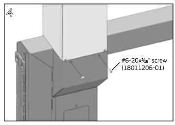
Install router cover per step 5 of the Vertical Utility Chase Housing instructions. Then secure extender cover to router cover with (2) #6-20x3/16" Phillips pan head screws.
