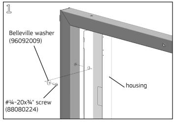
Align the large holes in the 2" side of the housing channel with the threaded inserts on the inside of the UltraFrame tube. Fasten housing to frame at the top and bottom with (2) ¼-20x¾" socket button head screws and (2) Belleville washers using a 5/32" Allen wrench.
