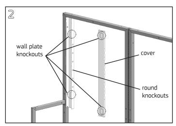
Remove knockouts as needed in housing channel and housing cover as necessary; install utilities.
