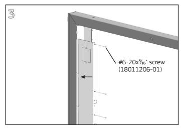
Align tabs on cover with slots in the short flange of the housing. Slide cover into slots and align holes in the cover flange with the holes in the housing. Fasten cover to housing with (9) #6-20x¾6" Phillips pan head screws using a #2 Phillips screwdriver.
