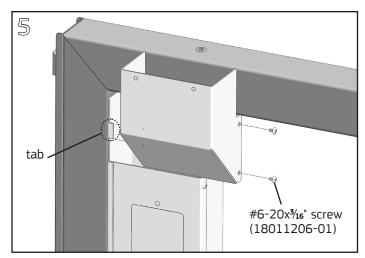
Align slot in the side of the routing cover with the tab on the routing housing. Slide routing cover over tab and fasten with (2) #6-20x<sup>3</sup>/16" Phillips pan head screws using a #2 Phillips screwdriver.
