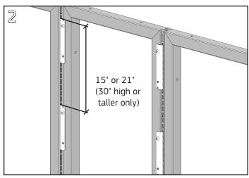
Install a hanger clip on the left and right side of the frame or panel with the screws at the top of each clip. The top of the Drain Board will be 2¾" above the top clip for 18", 30" and 36" high boards. The top of a 24" high Drain Board will be 5¾" above the top clip. For 30" high Drain Boards, install a second set of hanger clips 15" below the top set. 36" high Drain Boards will require a second set of clips 21" below the top set.
