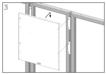
Align the large holes in the back panel of the Drain Board with the screws in the clips. Slide the panel down over the screws to engage.
