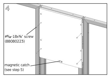
Install an additional 5/16-18x3/8" Phillips pan head screw into the bottom of each hanger clip. Fully tighten all top and bottom clip screws with a #2 Phillips screwdriver.
