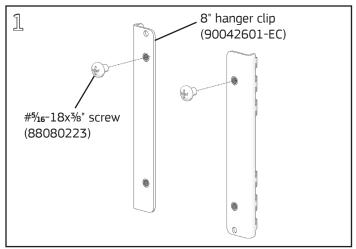
Install a 1/16-18x3/8" Phillips pan head screw into the top of each hanger clip. Leave a 1/8" gap between the screw and clip. For Drain Boards 30" high and taller, two pairs of hanger clips are provided.
