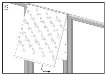
Install pegs in the Drain Board front panel. Hook the top flange of the front panel over the top of the back panel and rotate the bottom of the front panel down until the magnet catches at the bottom.
